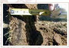
In response to the poor conditions, a custom soils amendment program was developed and implemented. This program included removal of the existing turf, incorporation of topsoil, compost, gypsum, sulfur, and specialized liquid fertilizers.
